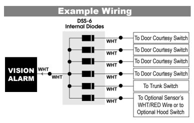
**NOTES**: The Door and Trunk pin switch connections are typically found at the body computer or fusebox inside the cabin. Some older vehicles still require running a separate wire all the way to the actual switch in the trunk. You do not have to connect all 6 wires shown above (e.g., if you have a 2 door car with a trunk, you only need 3 out of 6 -- leave the others disconnected.)
