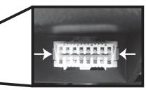
While pressing inward on the two tabs shown above by the arrows, push the factory OBD connector out the back of its slot.
