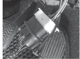
**NOTE.** A wire tie can be used as shown above to ensure the connectors won't ever pull apart.
