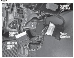
Attach your OBD device to the remaining **White** OB-22W connector as shown. (*The plug in the factory OBD slot is left open.*)
