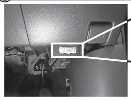
**NOTE.** The factory OBD on some cars may be mounted slightly different than the two photo above.
