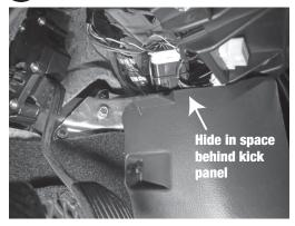
The above photo shows just one example of where to hide wires. Ensure your location does not interfere with the vehicle's moving parts.
