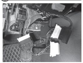
Attach your OBD devices to the remaining two white OB-23W connectors, as shown in the above photo example.
