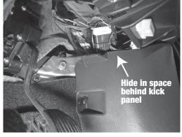
The above photo shows just one example of where to hide wires. Ensure your location does not interfere with the vehicle's moving parts.
