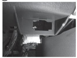
Select any one of the 3 white OB-23 connectors to insert into the factory OBD slot. (Normally you would use plug C.)
