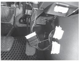
**NOTE.** The above photo shows the OB-23W connected, with White plug C mounted in the factory OBD slot.
