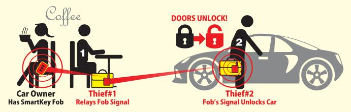
Many modern car security systems use the keyless entry system to Arm on door Lock and Disarm on Unlock. A Relay Attack could allow a thief to Disarm your car's security system!
